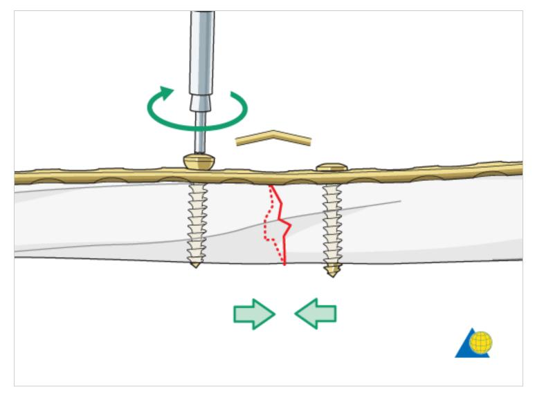
Tighten both screws alternately, watching carefully to see that the reduction is maintained and compressed satisfactorily.
