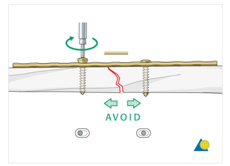
When a transverse or short oblique fracture is compressed with a plate, this eccentric plate compresses the bone under the plate, but causes gapping on the side opposite the plate (trans cortex). This gapping, and its consequent associated micromotion, can be prevented by overbending the plate to achieve compression of the opposite side first.
