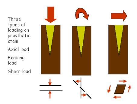
When a hip prosthesis is implanted in bone the bone-stem or bone-cement-stem becomes a composite structure. Although bone makes up most of the mass of the composite, the metal stem because of its high stiffness compared to bone takes up most of loading. This requires an understanding of some basic principles of composite loading
